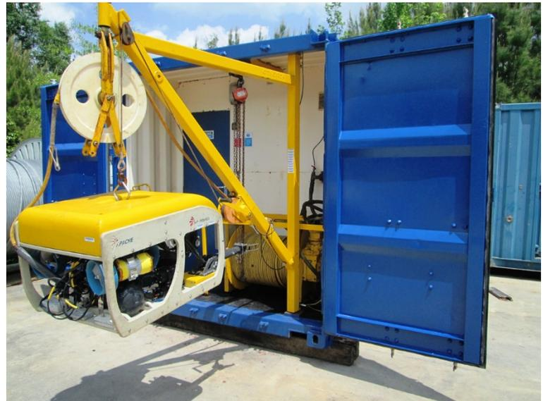
**The OTS - Apache Inspection Class ROV offers a truly versatile, professional ROV system suitable for offshore use. Its compact size provides a suitable platform for high quality video and sonar surveys all within a single lift container.**
